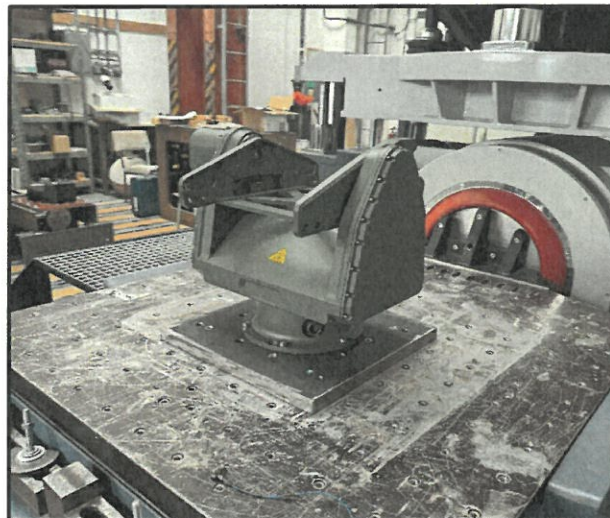
Figures 4, 5: EUT (X test axis orientation)
