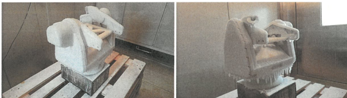
Figure 4 Tested device after the required ice layer is formed
