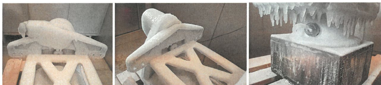
Figure 5 Detail of the EUT with a layer of ice
