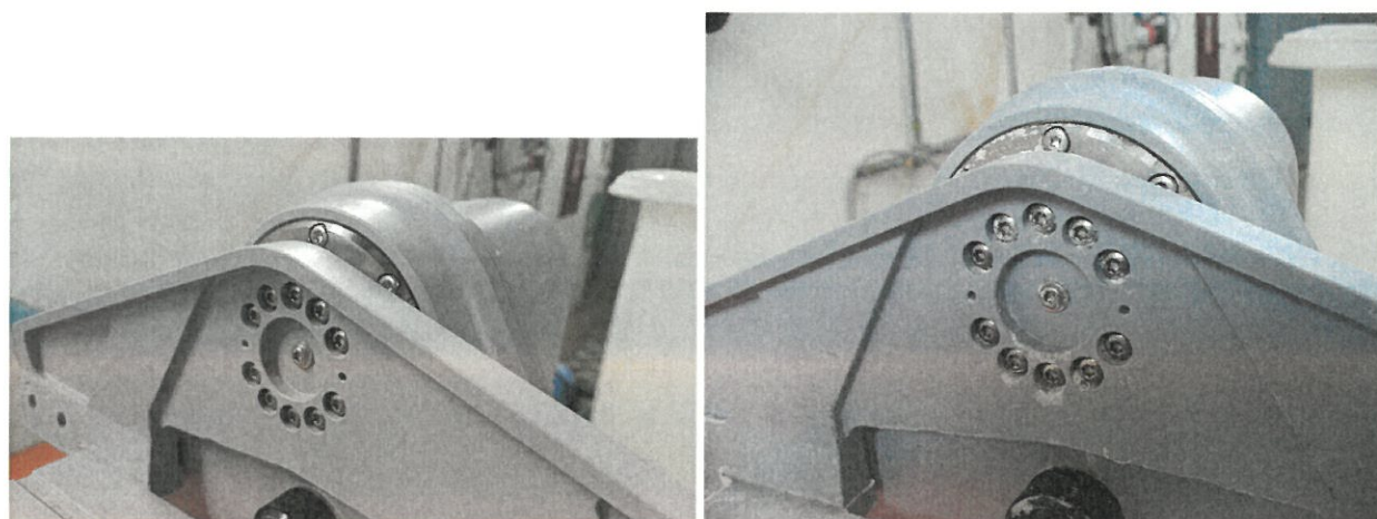
Figure 5 Detail of the platform attachment (left – before the test, right – after the test)
