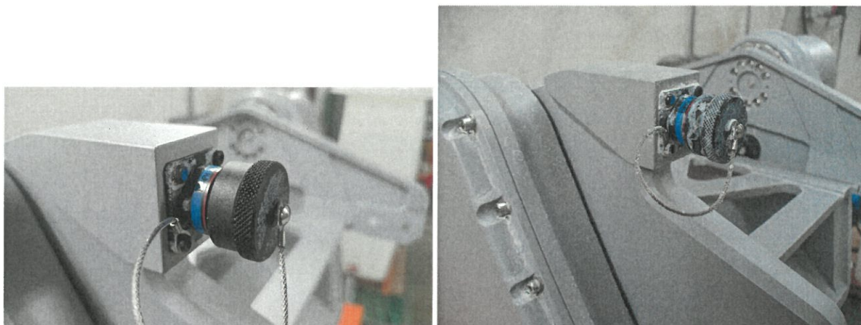
Figure 3 Detail of the connector on the platform (left – before the test, right – after the test)
