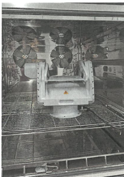
Figure 2 Placement of tested devices in the climate chamber ClimeEvent C/1500/70a/5
