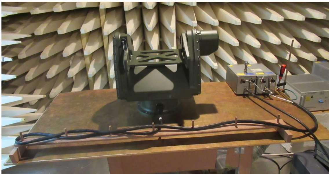
Figure 2.1.A – EUT during conducted emissions test
