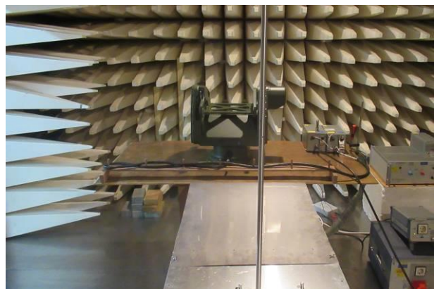
Figure 2.2.B – EUT during radiated emissions test
