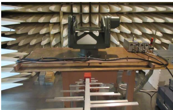
Figure 2.2.A – EUT during radiated emissions test
